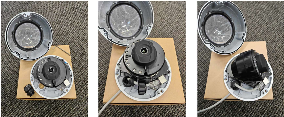
Figure 2: Installation of PoE cable
